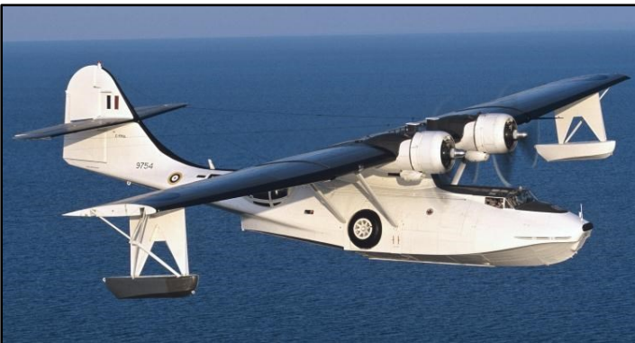
The PBY Canso, on which WO2 Leatherdale flew as a flight engineer, was an amphibious version of the PBY Catalina. The retractable wheels can be seen on the side of the fuselage.
